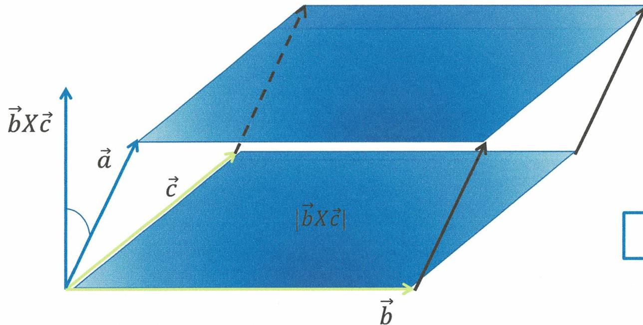
$$[\vec{a} \vec{b} \vec{c}] = \vec{a} * (\vec{b} \times \vec{c})$$
